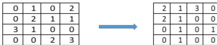
Figure 4 Example of GLCM calculation in the horizontal direction and using offset 1 pixel.
