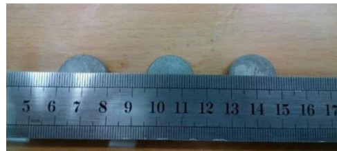
Fig. 4.1: Showing prepared composites samples after sintering and Heat treatment.
