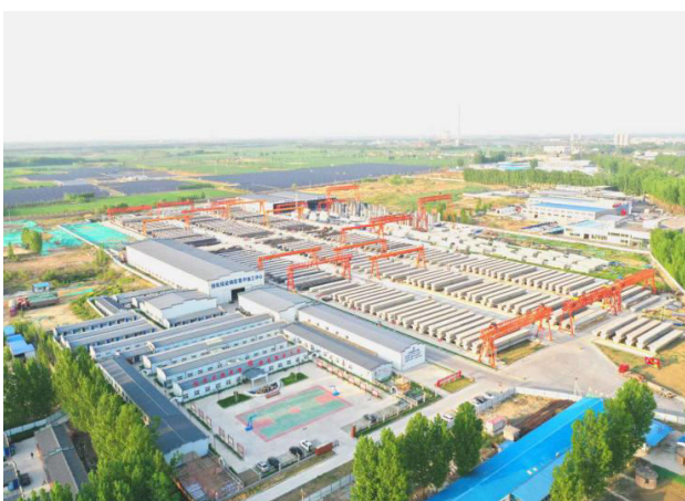
Fig. 3 The green construction technology—prefabricated bridge construction (a) The standardized centralized prefabrication of components in the precast factory (b) The on-site hoisting, installation, and connection of prefabricated components
