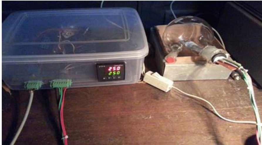
Figure 5 : Experimental Set up of gas sensing measurement system
