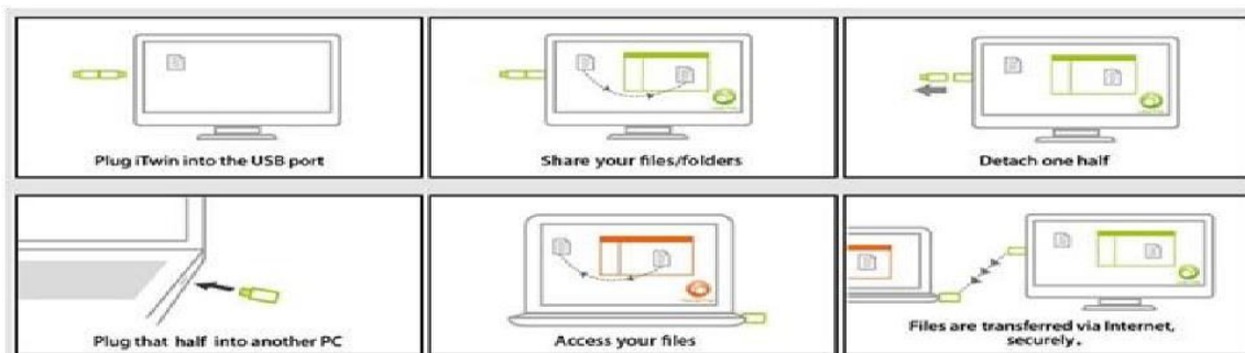
Fig 1 Working of iTwin
