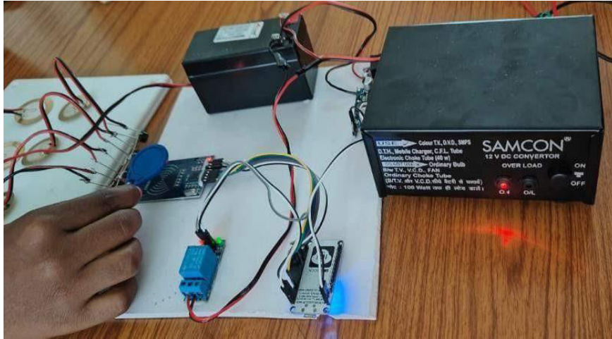
Fig.5: Developed model of footsteps power generation using piezoelectric material
