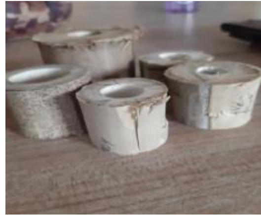
Fig.6. Vertical crack failure of the specimen after compression test.
