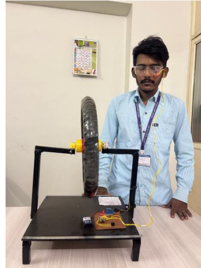
Figure 15: Close Eye Position (Yellow & Red Light ON in Eye Blink Sensor)
