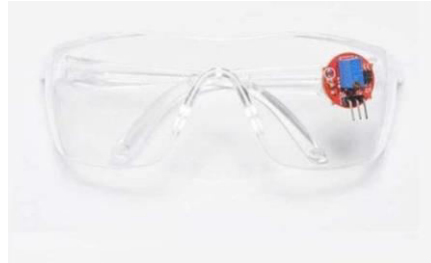
Figure 5: Eye Blink Sensor
