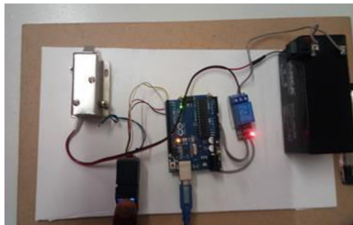
Fig 5.3 Smart Finger Print unlock System (lock closed)
