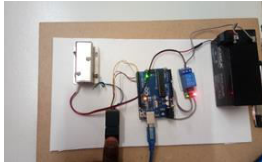
Fig 5.2 Smart Finger Print unlock System (lock opened)
