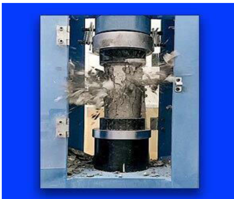
Fig.14: testing cylindrical concrete specimen.
