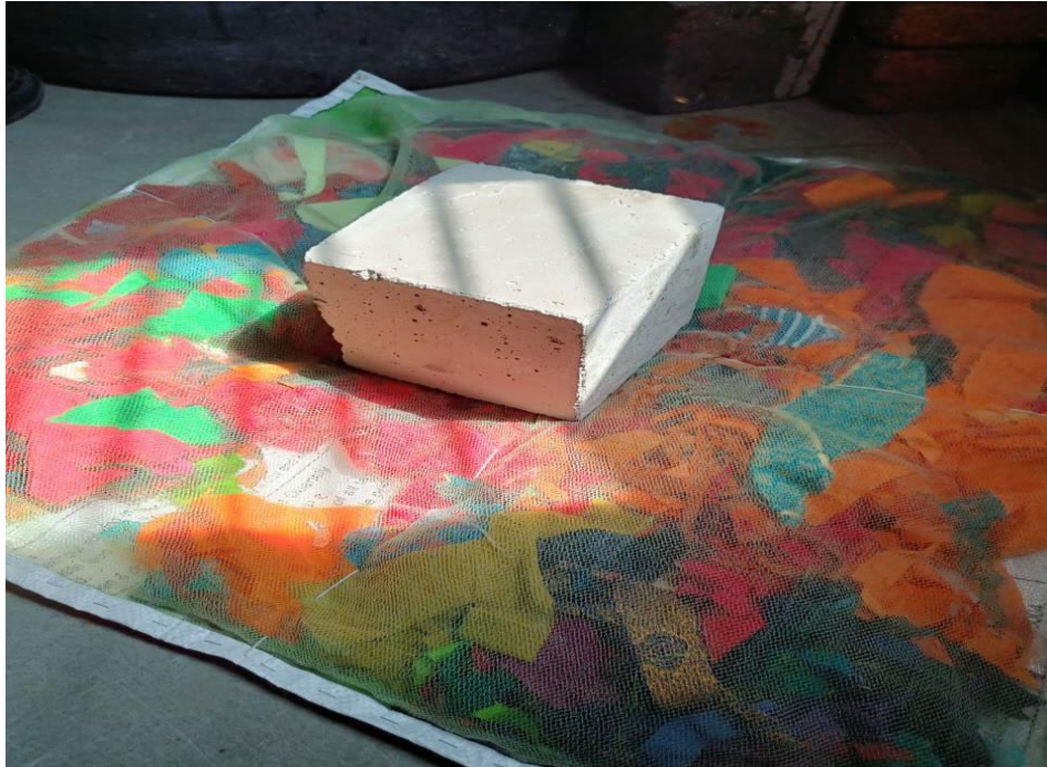
Fig 12. Efficient curing pad for curing to concrete.
