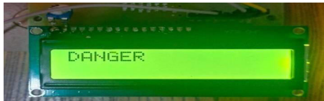
Fig4.4Scenario shows the danger condition when below the 10cm
