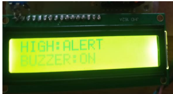
Fig(b): "High alert": Buzzer activates upon human activity detection. Audible alert signals heightened vigilance and potential security risks
