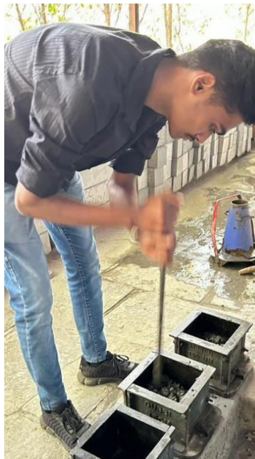
Fig.5. Compacting Using Tamping Rod
