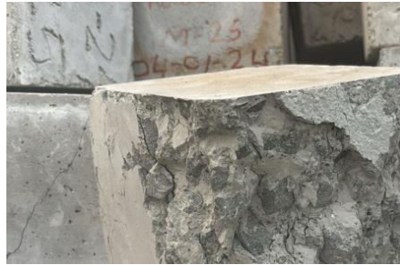
Fig.10. Damaged Cube (Sample 1)
