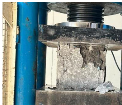
Fig.8. Sample Under Compressive Strength test
