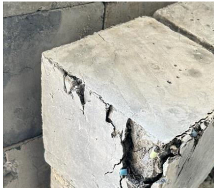
Fig.11. Damaged Cube (Sample 2)
