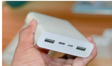
Figure 5. DC power bank
