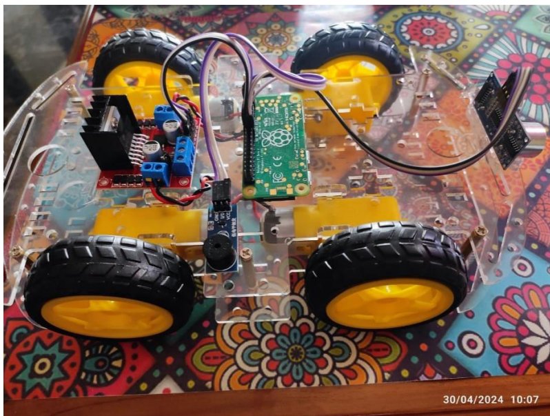
Fig 2: IOT-enabled Wheelchair navigating through eyeball movement
