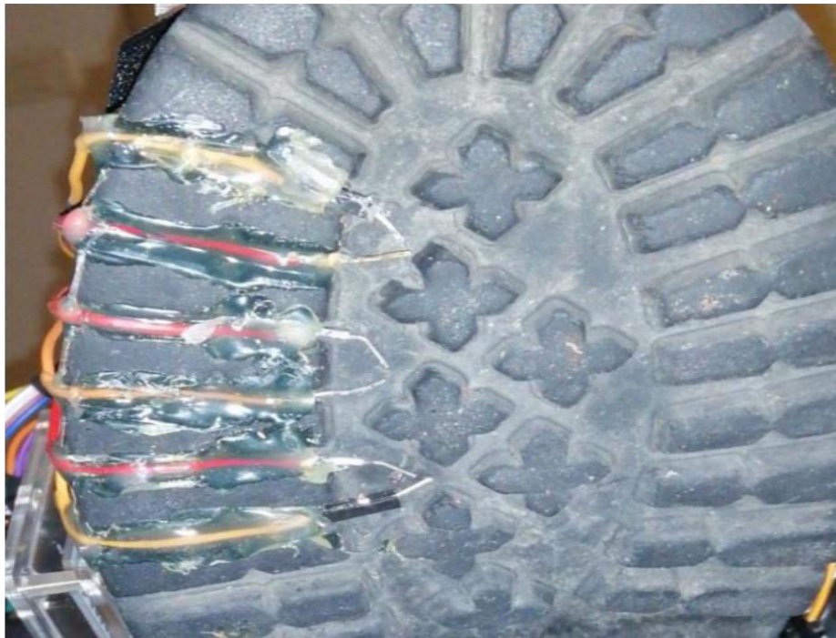
Figure 2. Placement of the wet floor sensor wires on the shoes
