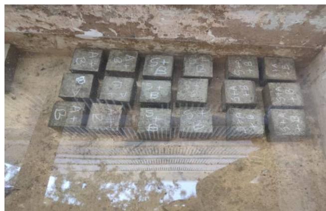
Curing of casted cubes
