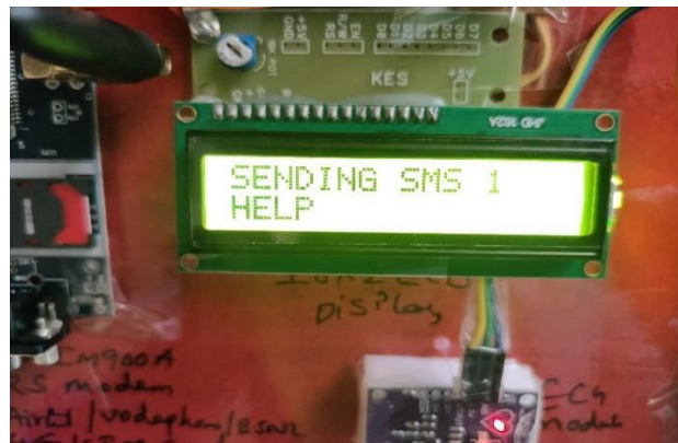
Fig 12: Output display for bending fore finger and middle finger at a time
