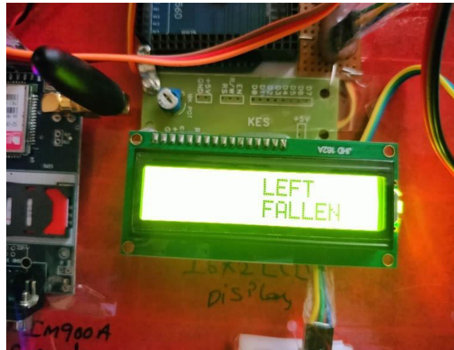
Fig 14: Output display for accelerometer input
