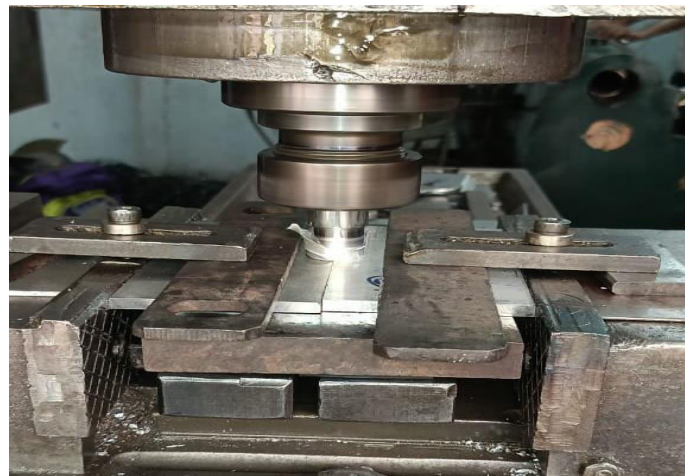
Figure 1 Friction stir weld on the dissimilar aluminium metal alloy
