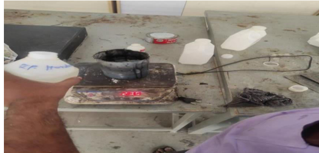
Figure 3.5 Prepare the EPOXY(250g to 280 g)/plate, Hardner 10%/plate and Mansion Wax Polish
