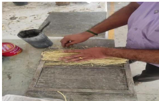
Figure 3.8 Cut the fiber length upto 30cm
