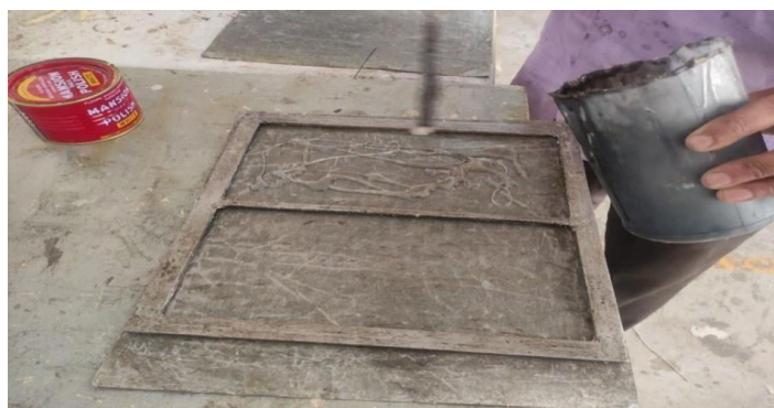
Figure 3.9 (a) Apply the Epoxy Resin in working plate
