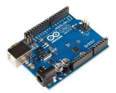
The Arduino Uno is a popular microcontroller board used in electronics projects and prototyping. It is based on the ATmega328P microcontroller and is known for its ease of use, versatility, and extensive community support. Here are some key features and specifications of the Arduino Uno:
