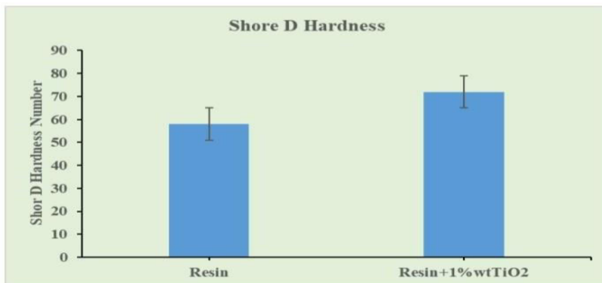
Fig. Effect of Titanium oxide filler on hardness
