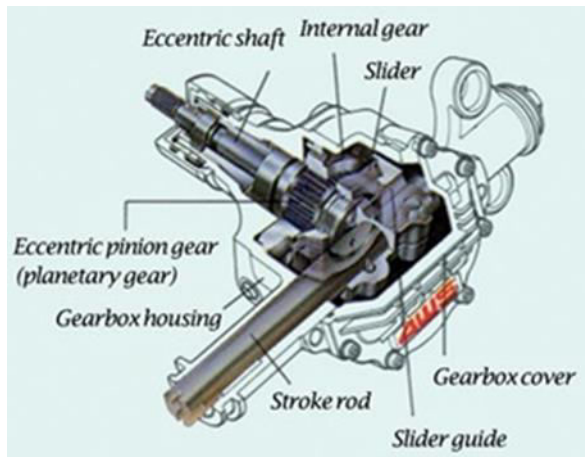
Fig. 5. 4WS mechanism (Honda)
