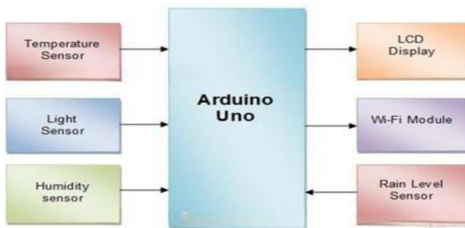
fig.1 block diagram of weather logger with education and research
