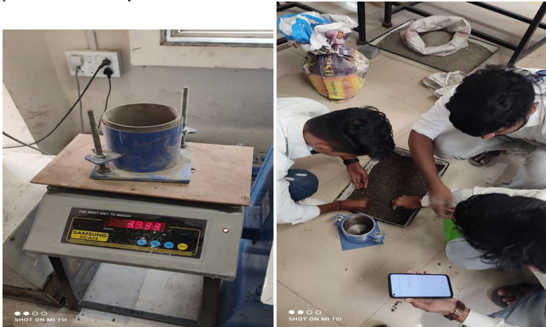
Fig no. 3: Standard proctor test for soil – fly ash mixture
