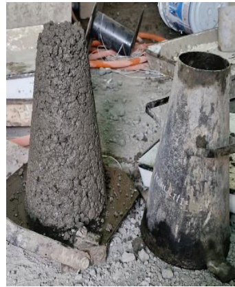
Fig no. 3 (Slump cone).
