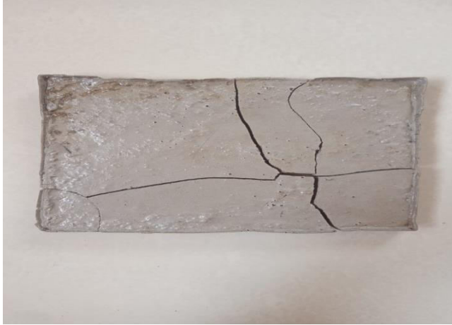
SAMPLE 7 FLY ASH + POND ASH + PLASTIC (1:2.2:5)
