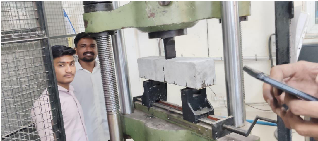
Fig No 4.2 Flexural test on Strengthened beam.
