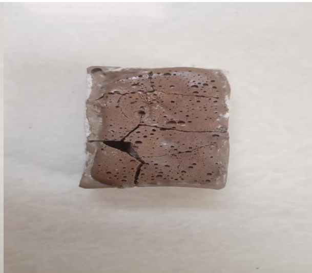
SAMPLE 4 CEMENT + FLY ASH + PLASTIC
