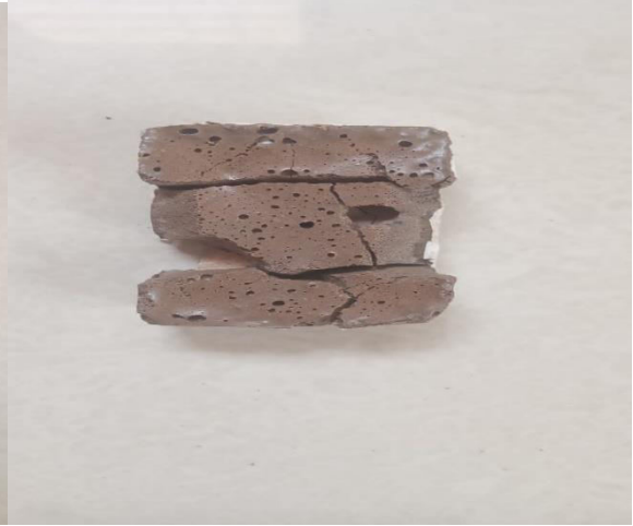
SAMPLE 2 CEMENT + FLY ASH + PLASTIC
