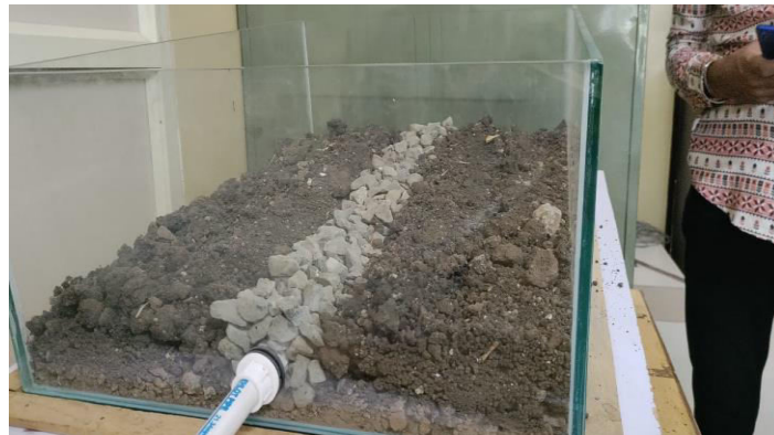
Fig 6 2 nd Layer till root zone with diged trench in it
