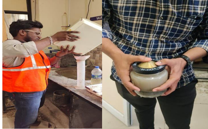
Fig 2. Specific Gravity Test / Water Absorption Test
