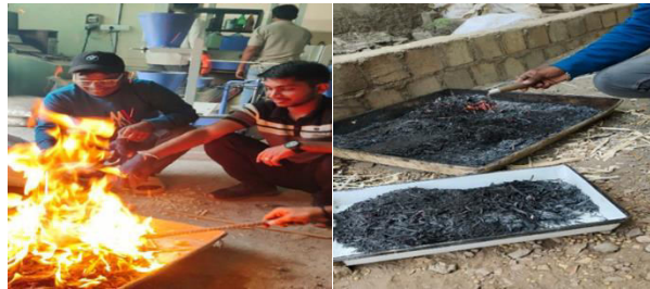
Fig 1. Burning Process Of SCBA
