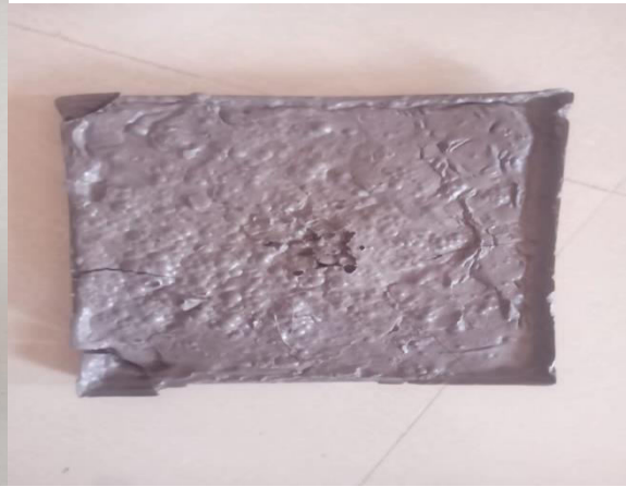
SAMPLE 8 FLYASH + FINE AGGREGATE + PLASTIC (1:1.5:2)
