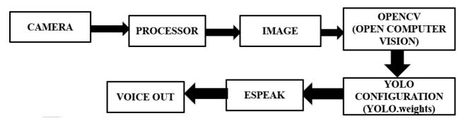
The camera takes a picture, and sends it to the processor along with the estimated data. The pictures taken by the camera and recognized can be checked by the processor for identifying objects around individuals as shown in block diagram.
