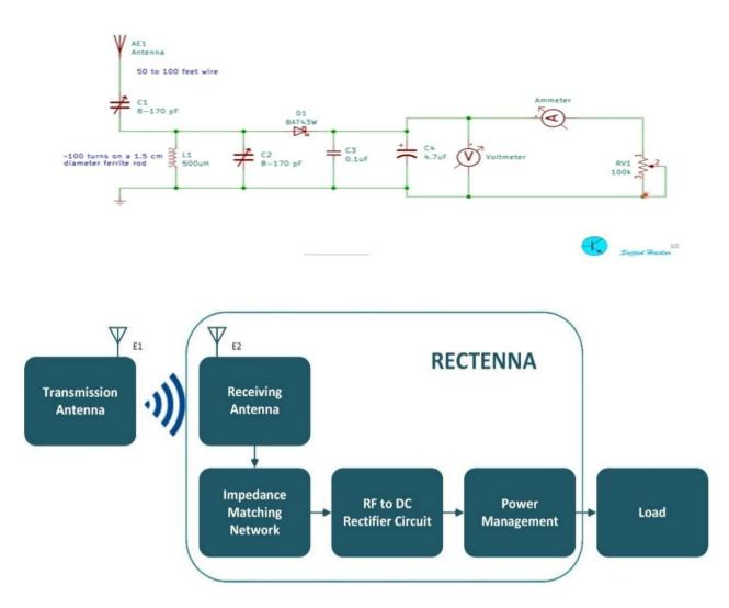
This diagram illustrates the energy harvesting process from ambient radio frequency (RF) signals using a rectenna system. Here's a breakdown of each component and its role:
