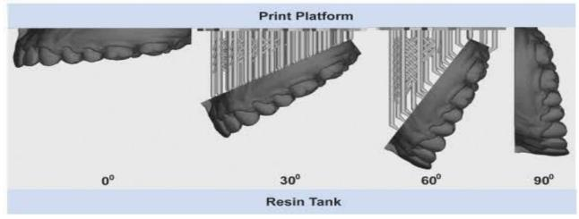
**4.5 Deposition Speed:** The speed at which material is deposited affects layer adhesion; finding the right speed is crucial for good structural integrity. In 3D printing, part orientation refers to how the object is positioned on the print bed during the printing process. It plays a crucial role in the quality, strength, and print time of the final part. Here are the main factors to consider when deciding on part orientation:
