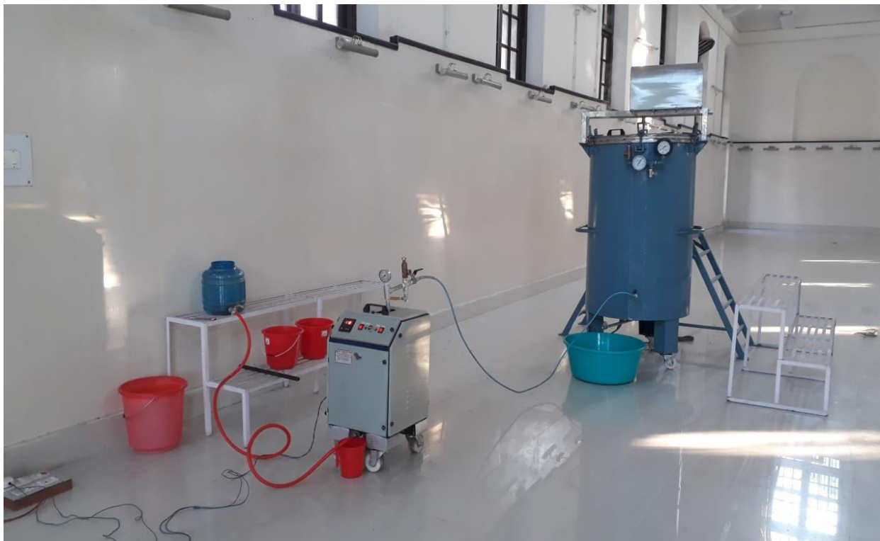
Fig. 1. Modified Steam Explosion Treatment Machine (MSETM) was developed by ICFRE- Forest Research Institute, Dehradun, Uttarakhand, India
