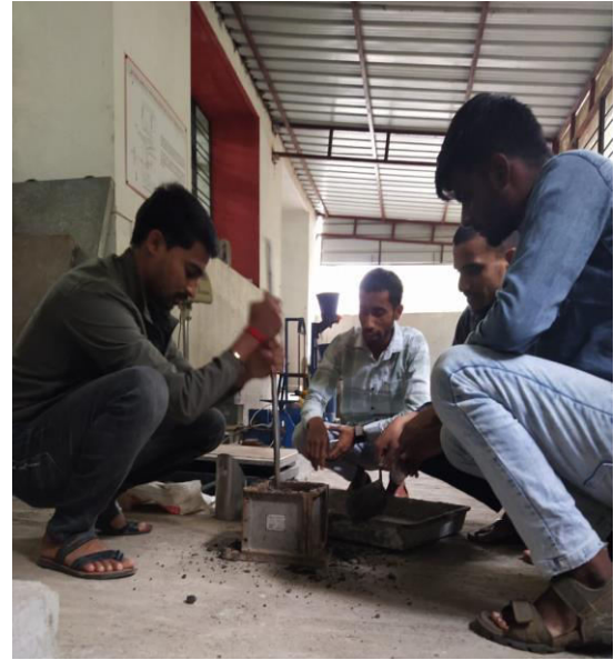
Fig 3.3.2 Dry mixing of materials
