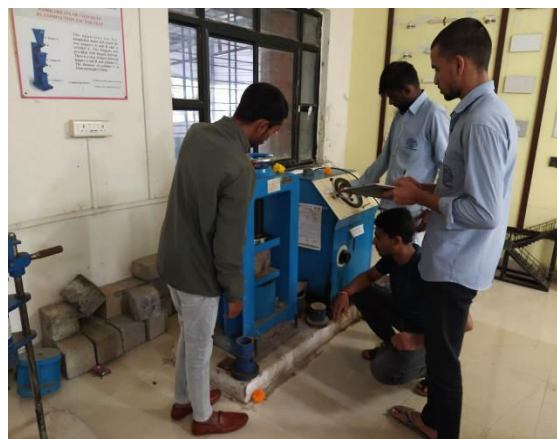
Figure 3.3.5 Compressive testing in CTM.
