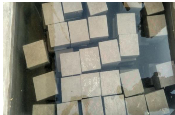
Fig. 3.3.4 Curing in Curing tank
