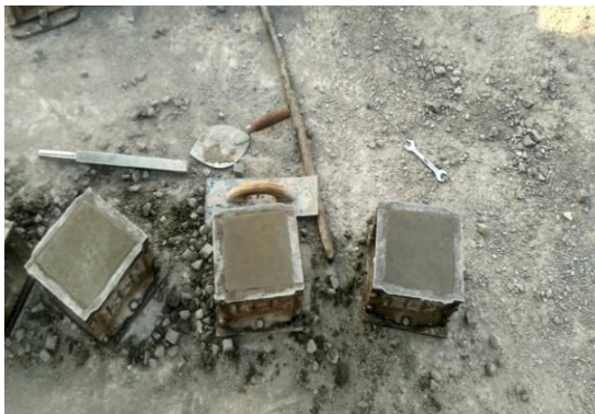
Fig. 3.3.3 Filled and finished cubes
