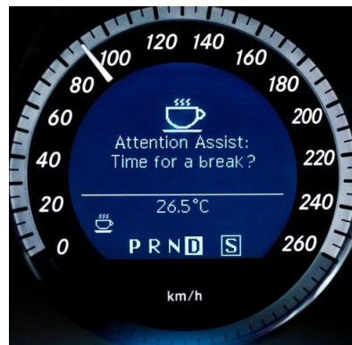
Figure 1: A speedometer from high-end cars illustrating how the alert message is displayed at regular intervals.
