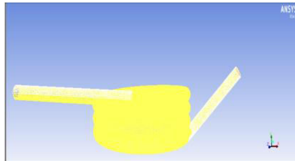
Figure: 6 FLUENT simulation model of Helical Coil N=3.25
