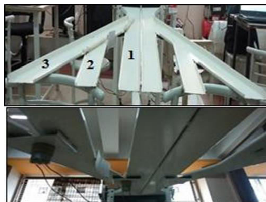
Figure No.3: Segregator system with DC motor and linkage
