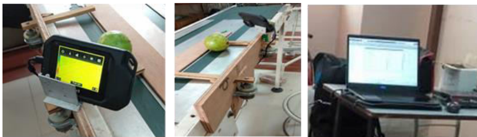
Figure No.2: Realtime Inspection of guava fruit and thermal images processed in MATLAB
