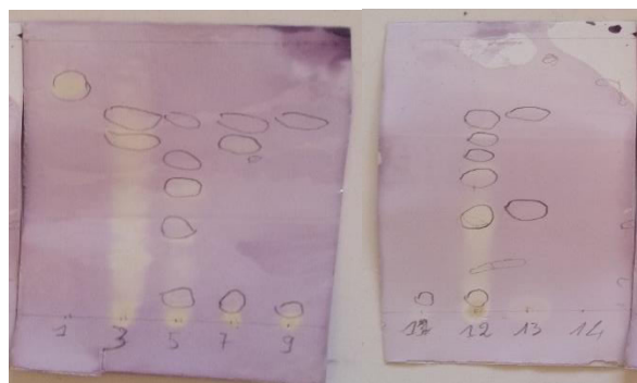
Figure 5 : TLC of the antioxidant test of crude extract fractions with ethyl acetate
