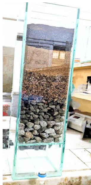
Fig 12. Experimental set up of filter media
