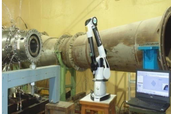
Fig.1 AACMM during inspection process
