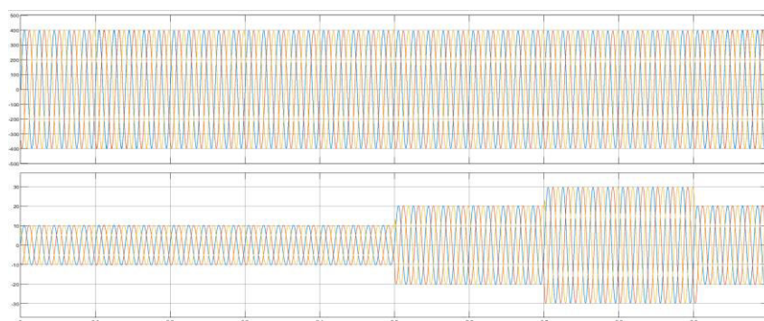
Fig. 3: Dynamic compensation waveforms of load voltage
