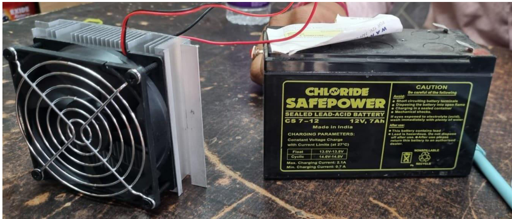
Figure 1. Mini Refrigerator with Battery (7V,12A)
