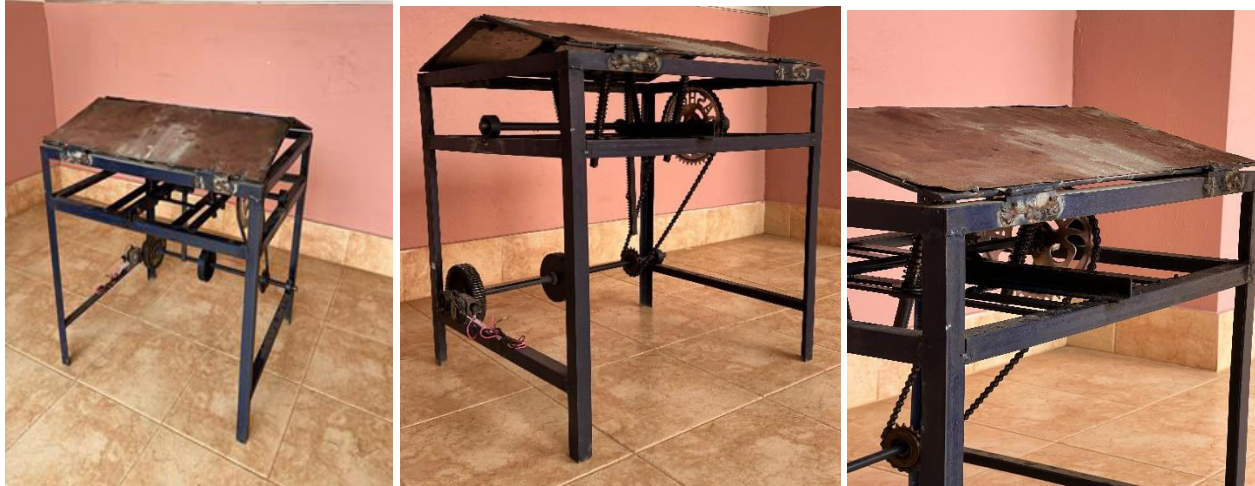
Fig.4 Fabricated Speed breaker electricity generator
