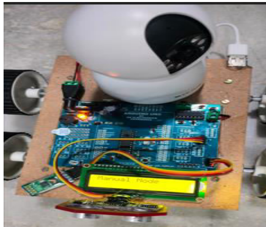
Fig. 12. Hardware setup model for manual mode
