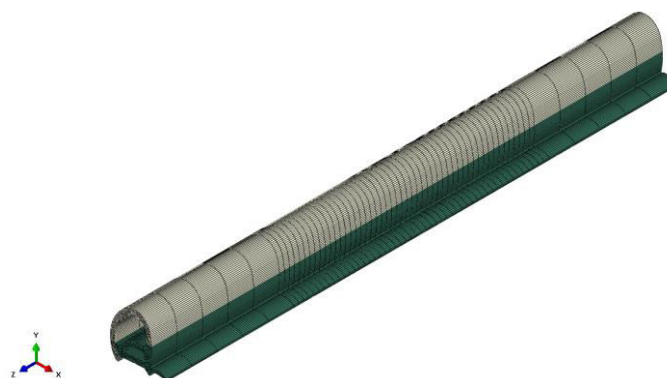
Figure 2. Weather strip seal – 3D mesh
