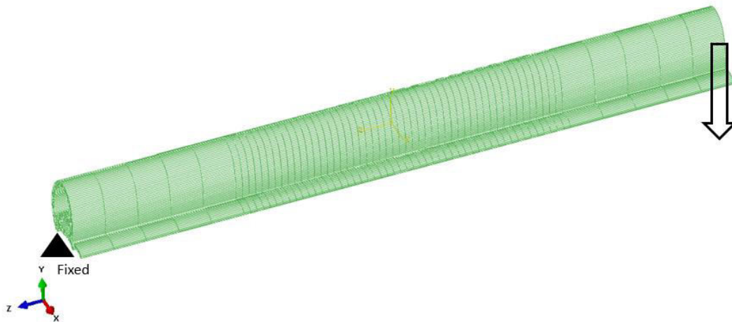
Figure 7. shows the finite element model of the weather-strip seal for a 3D analysis.
