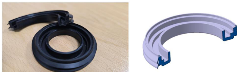
Figure 2. a. 3D CAD SEAL a. Full view, b. Section in detail view
