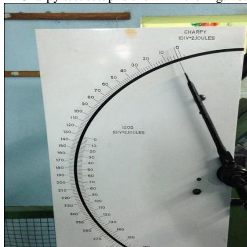
Fig. 10 Energy Reading after impact testing (2 J)
