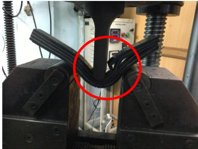
Fig. 8 Flexure Loaded Test Specimen
