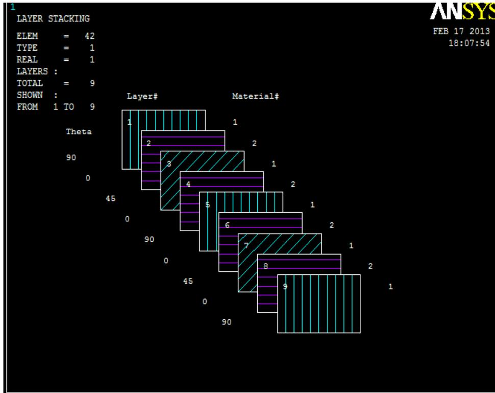
Fig. 2 Modeling of the CFRP in ANSYS
